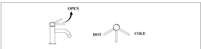
By lifting the Lever Handle upwards, the valve will be activated. Water flow will increase by continuing to lift up the Lever Handle. By rotating the Lever Handle counter-clockwise, the water temperature will decrease. By rotating the Lever Handle clockwise, the water temperature will increase.
